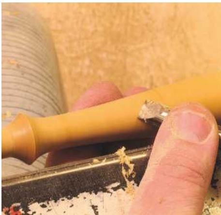
▲ Pic.31 After the initial shaping with the roughing gouge, use the 10mm skew to plane the handle. Because of the vibration, support the wood with your fingers behind the work
